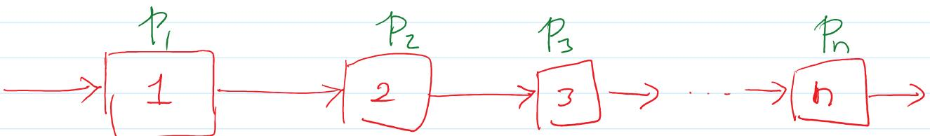
the prob. of failure at each subsystem is  $p_i$
